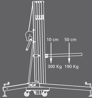
The TL-A320 can lift 320kg with the centre of gravity situated at 50cm from the towerlift profile. This means that the front of the Line Array can be at 1 metre from the towerlift.
